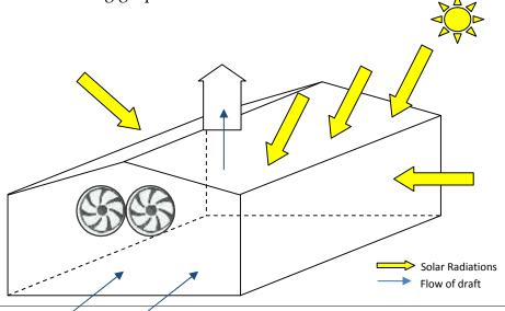
• The arrangement contains, as shown in the graphics, a tempered glass house with a churning machine inside to evenly distribute the coal in a layer of fixed thickness. Fans are arranged at the inlet side of the drying area to provide draft to the moist air. An exhaust chimney is provided for creating a suction draft inside the drying area.
